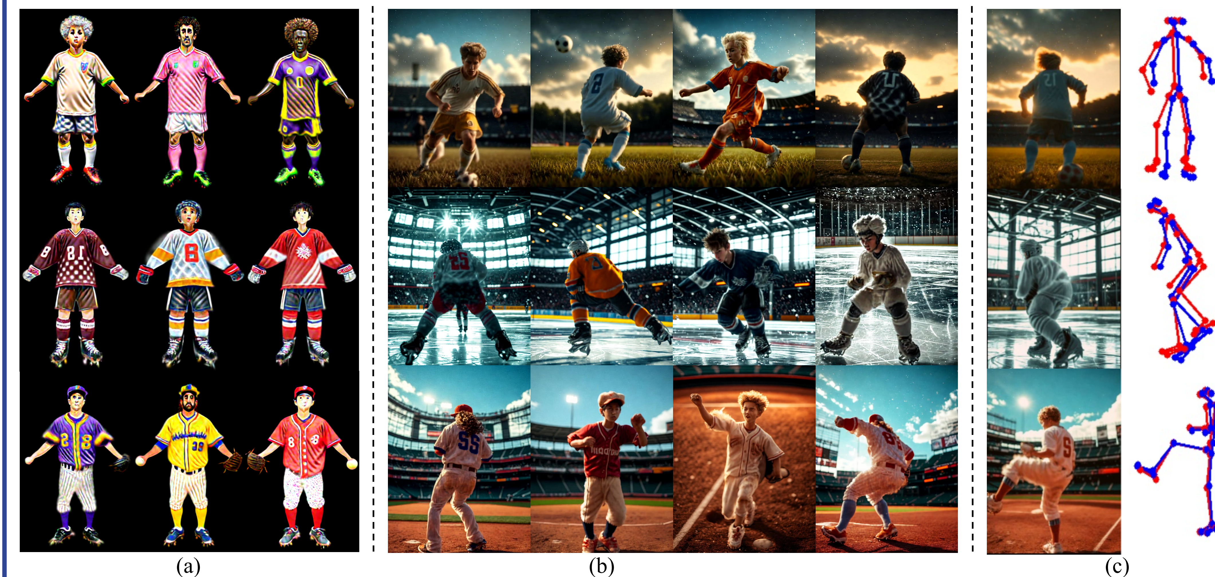
(a) Examples of 3D canonical avatar representations; (b) Final rasterized synthetic frames with avatar animation and pose-aware backgrounds; (c) Qualitative visualizations of pose estimation results trained on SportPAL using TokenPose [1].
